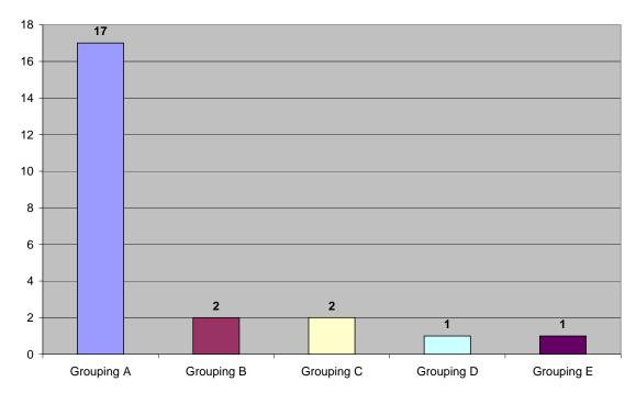
The 17 additional information reaching 70,8% of the total that point to stator winding damage (Grouping A) show that this is the most critical part of the machine and deserves special attention when the GFP's design is made.
