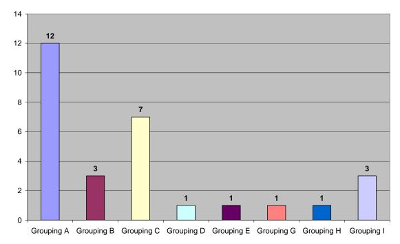
The result confirmed the preference for CO2 considered as most efficient extinguishing media by 12 Users, in second place water was indicated by 7 Users and Inergen got 3 favorable opinions (as a new media for hydro generators this is an interesting result).
